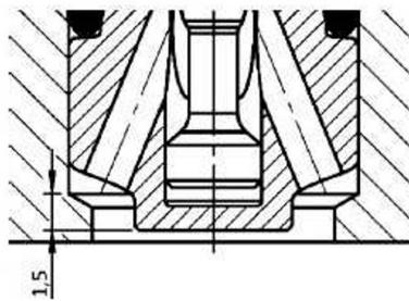
The nose of the valve protrudes by 1,5 mm into ID 10 mm of the cavity.
