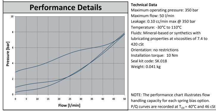
Maximum operating pressure: 350 bar Leakage: 0.10 cc/min max @ 350 bar Fluids: Mineral-based or synthetics with lubricating properties at viscosities of 7.4 to
